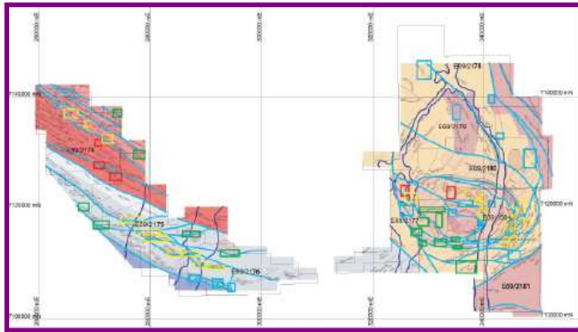
Fig 4: Geology and interpreted locations of faults and palaeochannels in the Warburton and Egerton areas.
