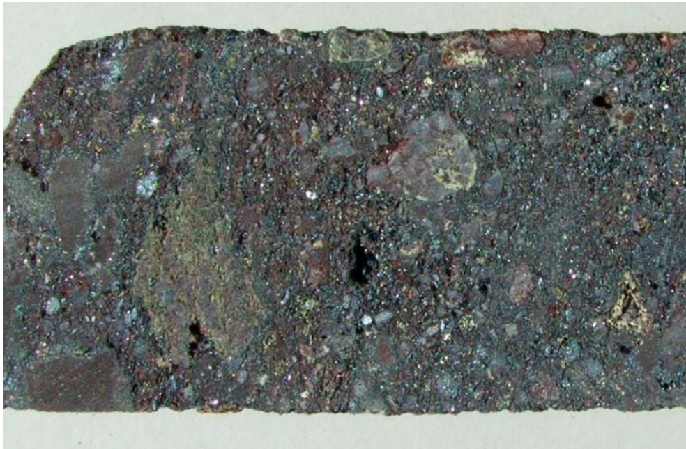
Figure 4: Detail mineralised section of drill core from MGD 047A
