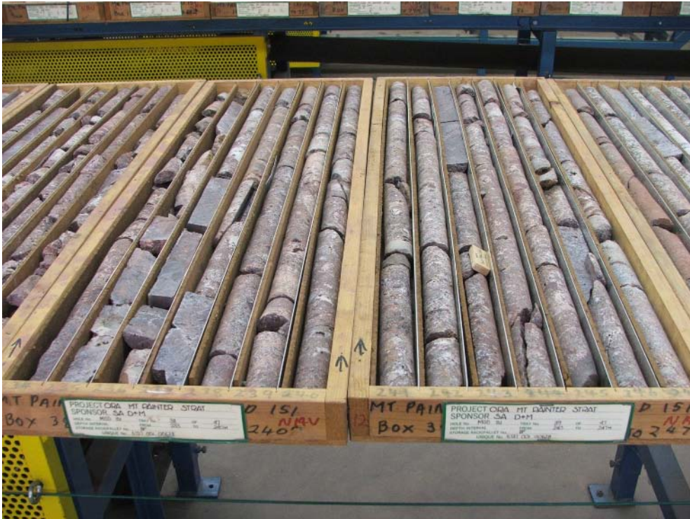
Figure 3: Drill core from MGD 151 showing mineralisation
